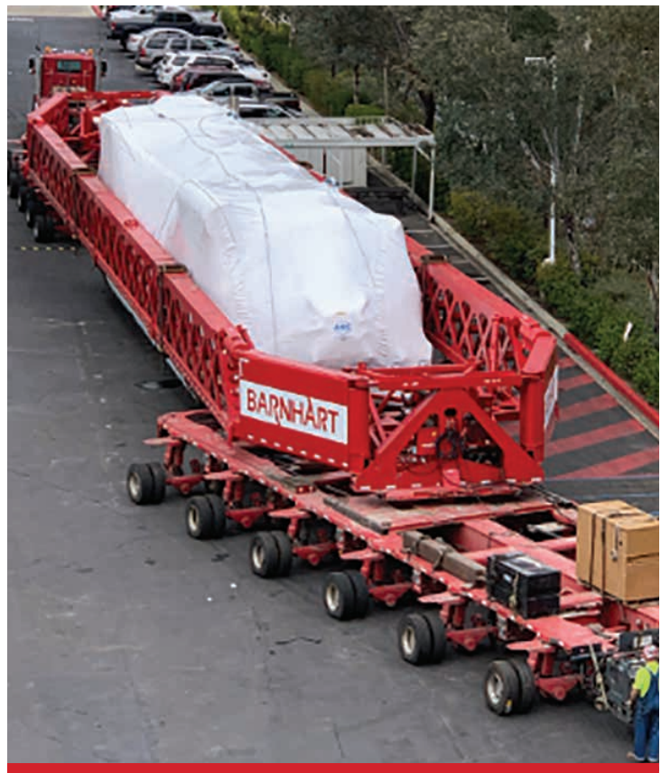
Aerospace: Barnhart hauls a 200,000-pound autoclave in its suspension girder system in Southern California.
